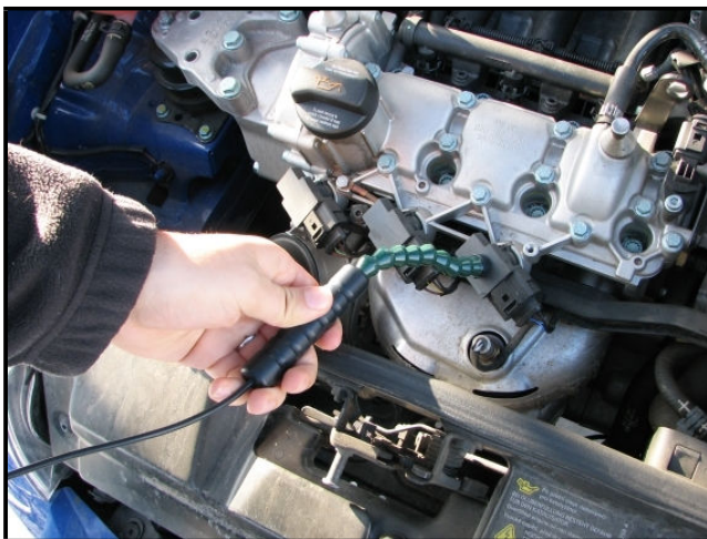
Demonstration of its use in the case of a simple comparison of HV courses between individual ignition modules
